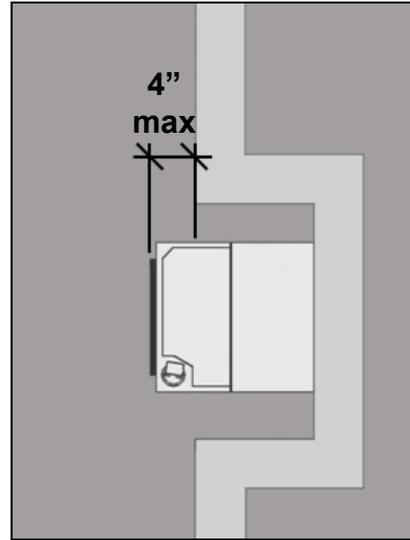
Elements, such as wheelchair accessible drinking fountains, must provide a knee clearance of at least 27". If located to provide, but not exceed this clearance (27" above the floor or ground absolute), they are not protruding objects because the leading edge will be within cane detection.
