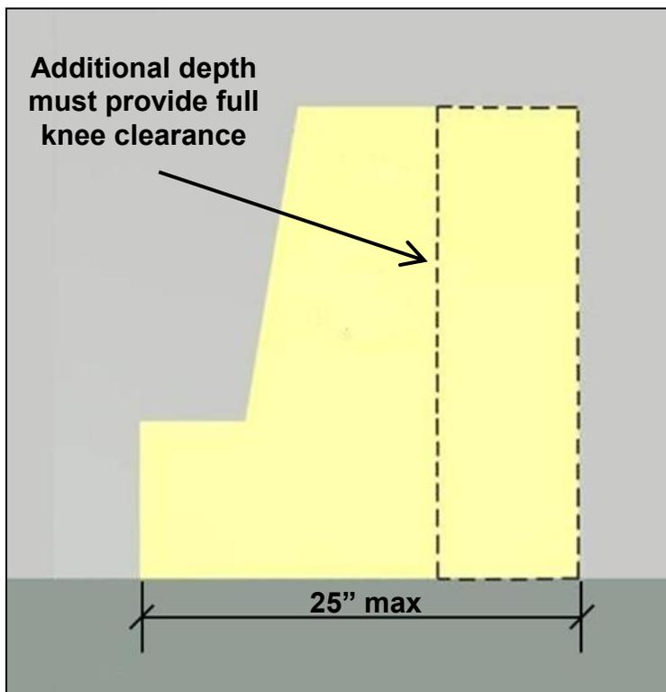
When the knee and toe depth exceeds the 17" minimum, the additional space must provide full knee clearance at least 27" high.
