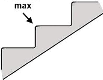
The radius of curvature at the leading edge of the tread must be  $\frac{1}{2}$ " max.
