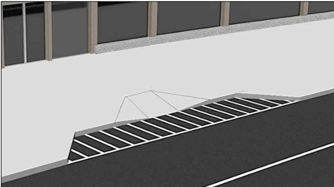
*At least 1 accessible passenger loading zone is required in every continuous 100 linear feet (or fraction) of passenger loading zone space.*
