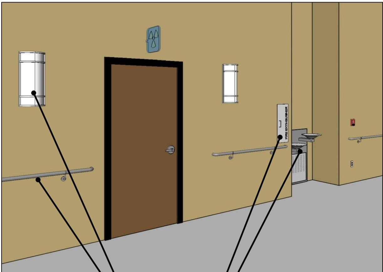
*Sconces, handrails, cabinets, drinking fountains and other elements that project into circulation paths must comply with provisions for protruding objects (unless they are located within cane sweep or above headroom clearance). Requirements for protruding objects apply to all interior and exterior circulation paths of sites. They are not limited to hallways and corridors and apply equally to circulation paths in rooms and spaces.*
