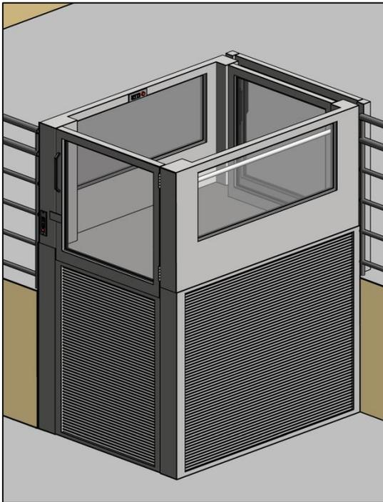
*The ASME A18.1 Standard specifies platform and runway enclosures for vertical platform lifts, among other features, and limits the travel distance. The size of platforms cannot exceed 18 sq. ft.*
