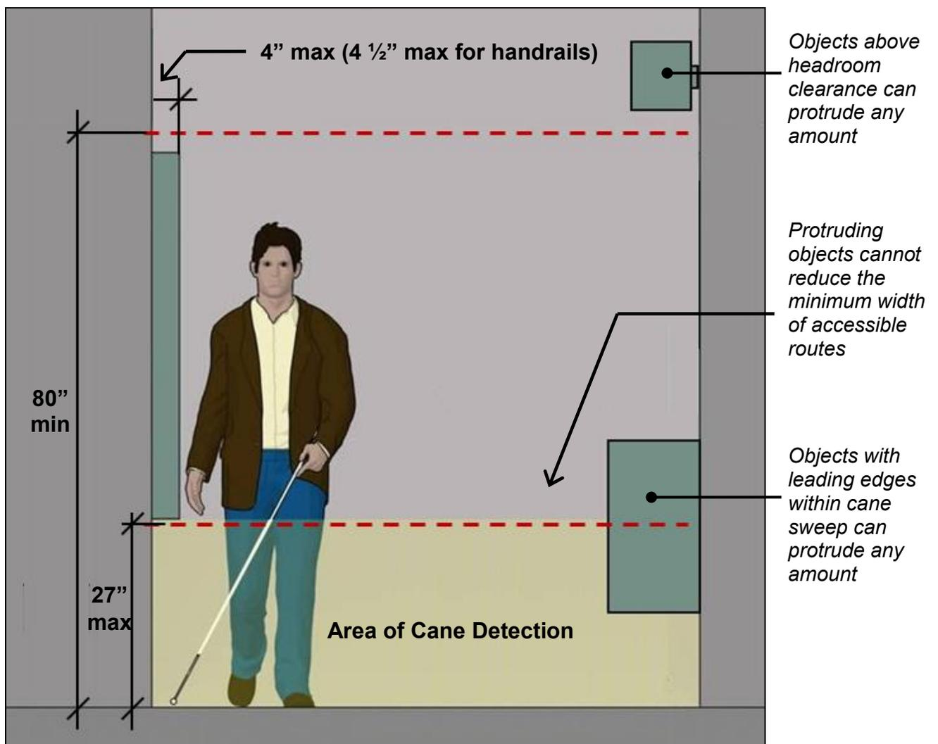
*Protruding object limits apply to the full width of circulation paths.*
