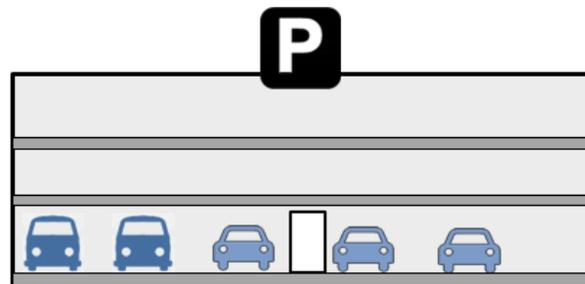
Accessible spaces, including van spaces, must be located so that they provide the same level of protection and security as other spaces in the garage. Locating accessible spaces required for a garage on the exterior is not usually acceptable.
