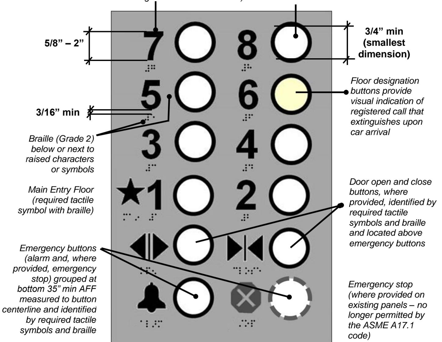
*In-car switches not for passenger use (e.g., fireman's operations) are not required to comply*
