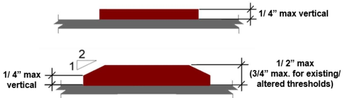
**Note: vertical edge must be located below bevel, not above**
