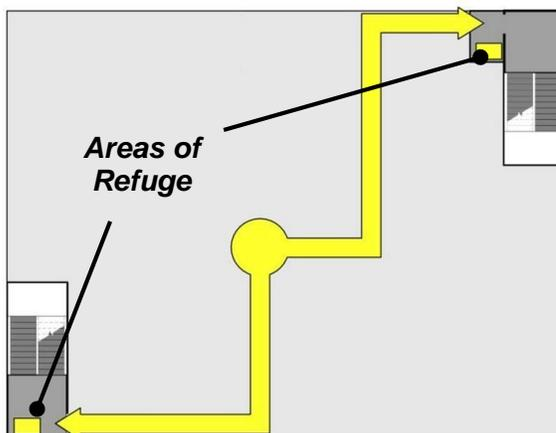
*Areas of refuge, which are required in buildings that are not equipped with sprinkler systems, provide fire and smoke protected areas where those unable to use stairs can register a call for help and await evacuation assistance. These areas must provide direct access to exit stairways and can be located adjacent to stairway enclosures or on stair landings outside the minimum exit width.*
