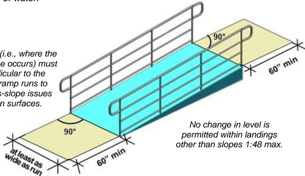
Intermediate landings between runs must be at least 60" wide clear and 60" long clear where ramps change direction (any change from linear). Handrails, edge protection, vertical posts and other elements cannot obstruct or overlap the minimum 60" by 60" clearance. The 12" minimum handrail extensions required at the top and bottom of ramp runs must be in the same direction of the run, but they can turn or wrap where handrails are continuous at the inside turn of dogleg or switchback ramps.
