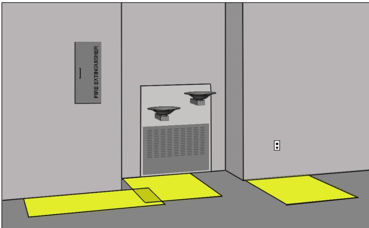
*Clear floor space is required at each accessible element, including storage cabinets, drinking fountains and other fixtures, and electrical outlets. Clear floor spaces can overlap where elements are in close proximity.*
