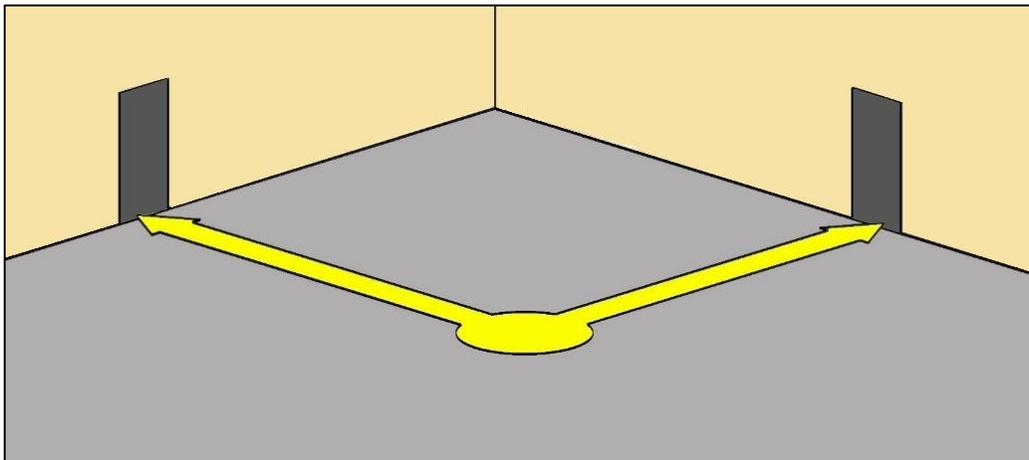
*Accessible means of egress can share a common path of egress travel as allowed for means of egress by the applicable building or life safety code (§F207.1).*
