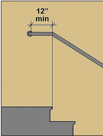
Handrails at the top of stairways must extend 12" minimum horizontally above the landing beginning directly above the first riser nosing or be continuous to the handrail of an adjacent stair flight (§505.10.2).
