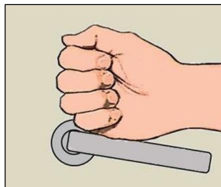
Hardware that can be operated with a loose grip or closed fist, such as lever-shaped handles and U-shaped pulls, accommodates the greatest range of users. (Closed-fist operation, while advisable, is not mandated by the Standards). Round door knobs do not comply because they require twisting of the wrist.
