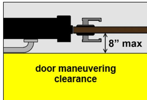
*Handrails and other elements cannot overlap the door maneuvering clearance but can be located within the 8" max. offset from the face of the door.*
