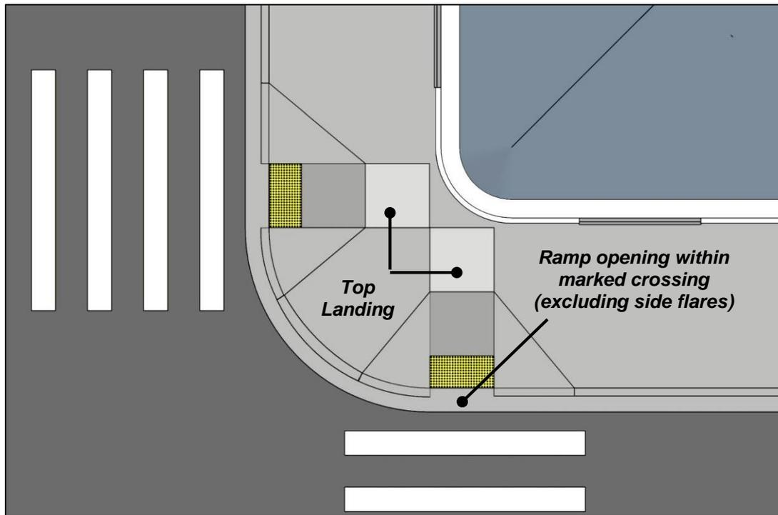
Curb ramps must be oriented so that the grade break is perpendicular to the curb ramp run to ensure a smooth transition to streets, including at corners with a wide radius. The curb ramp opening can be aligned with the curb line (left) or more directionally oriented to the crosswalk (right).
