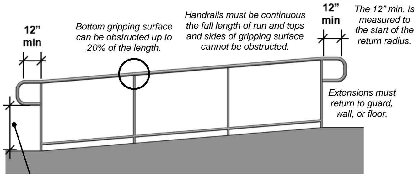
Extensions with a leading edge 27" high max. can extend any amount from posts. Those with a leading edge higher than 27" are limited to a 12" protrusion from posts (§307.3). The sloping portion of handrails are not required to comply with requirements for protruding objects.
