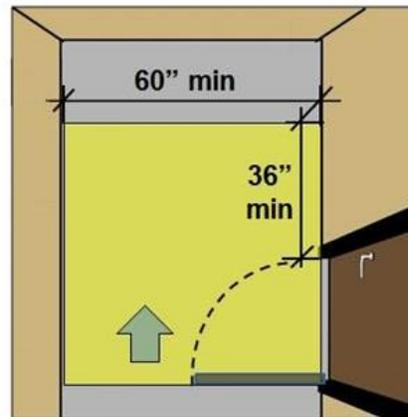
*On the pull side of hinge approaches, 36” min. latch-side clearance is required if the depth is 60” min. (The depth can be 54” min. if the latch-side clearance is at least 42”.)*
