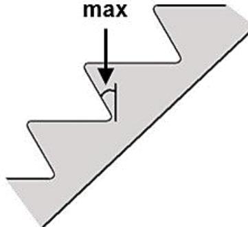
Risers can slope under the tread at an angle not exceeding  $30^\circ$  from vertical.
