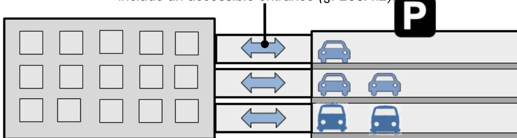
*Dispersing accessible spaces among accessible entrances requires placement of non-van accessible spaces on different levels. All van spaces can be grouped on one level (§F208.3, Ex. 1).*
