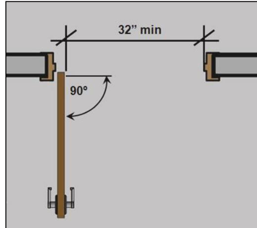
**Clear Width and Vertical Clearance of Doors and Gates [§404.2.3]**
