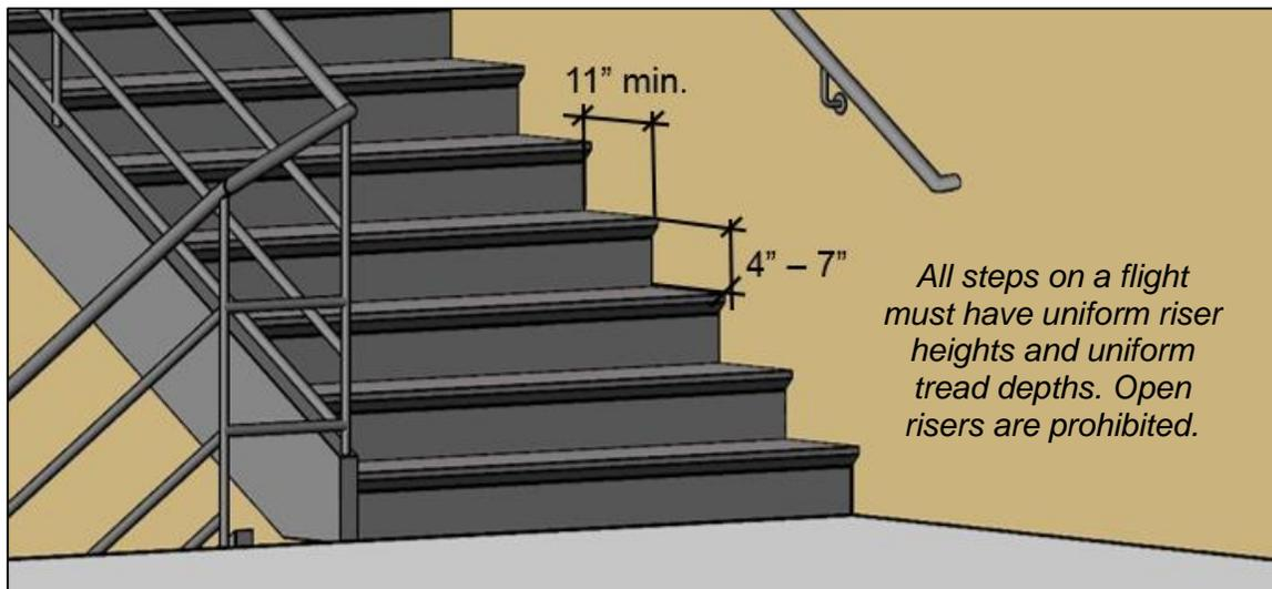
*Treads and landings subject to wet conditions must be designed to prevent the accumulation of water. Visual contrast on tread nosings or the leading edges of treads is helpful for people with low vision but not required by the ABA Standards.*
