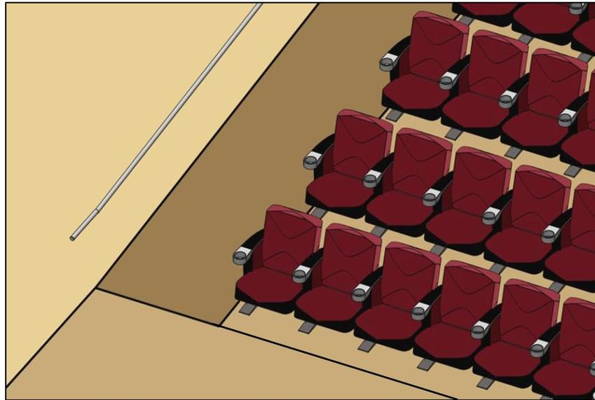
*Handrails on assembly area ramps can be discontinuous and lack extensions to allow access to seating and to permit crossovers within aisles. (§505.3, §505.10)*
