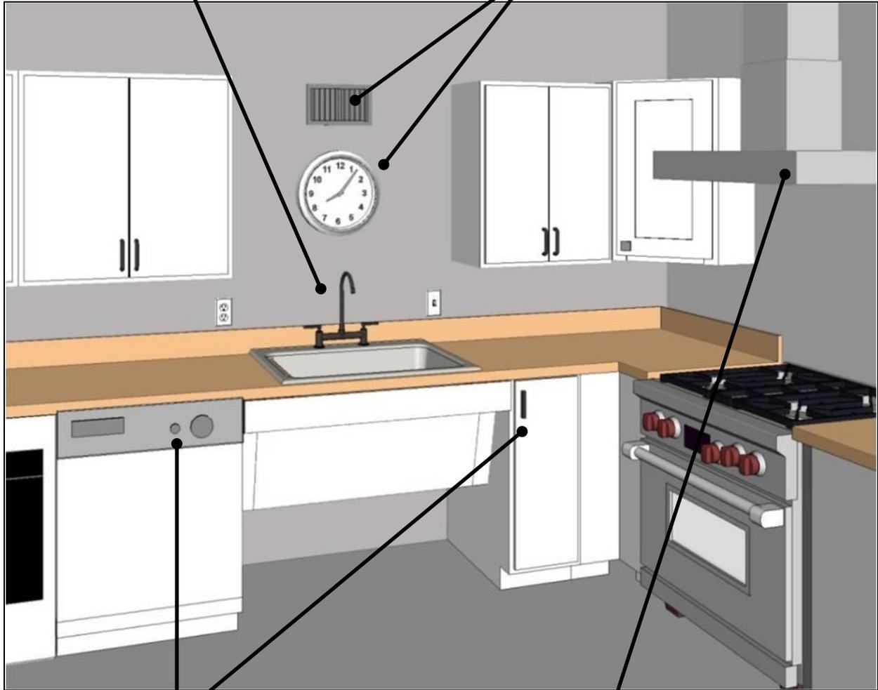
*Appliance controls and handles to accessible storage are also covered as operable parts.*
