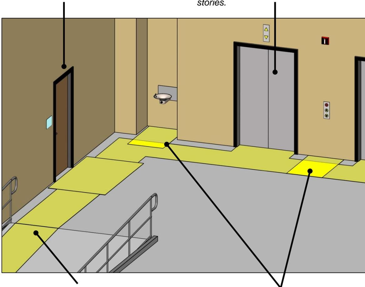
*Accessible routes must serve each level on a floor required to be accessible. Vertical access can be achieved by ramps, curb ramps, elevators or, where permitted, platform lifts.*
