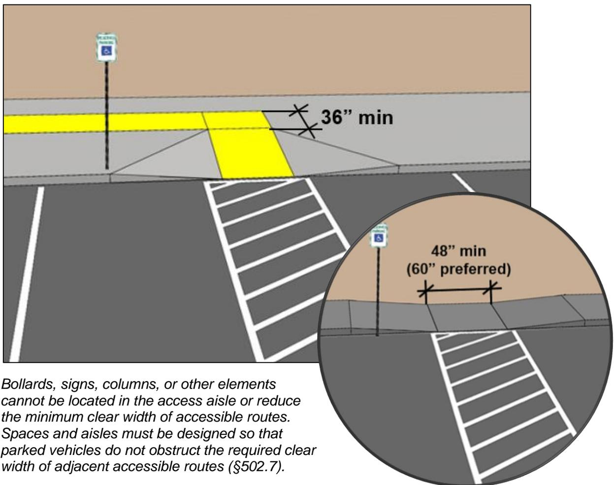
*Bollards, signs, columns, or other elements cannot be located in the access aisle or reduce the minimum clear width of accessible routes. Spaces and aisles must be designed so that parked vehicles do not obstruct the required clear width of adjacent accessible routes (§502.7).*
