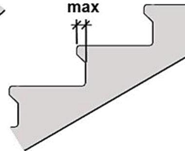
Nosings cannot project more than  $1\frac{1}{2}$ " over the tread, and the underside of the leading edge of the nosing must be curved or beveled.
