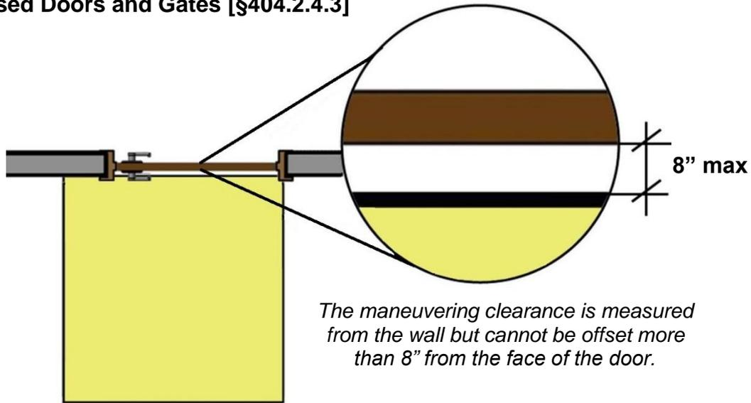
Thick walls, casework, shelving, columns and other elements can cause doors or gates to be recessed. If any obstruction within 18" of the latch side projects more than 8" from the face of a door or gate, maneuvering clearances for a forward approach must be provided. This space must be inset at obstructions so that it is no more than 8" from the face of the door or gate.
