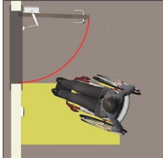
*Clear floor space at door control must be located outside door swing.*
