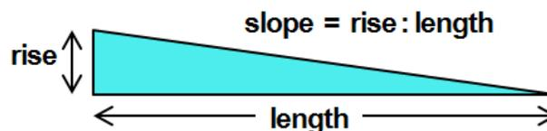
The running slope is to be uniform along a run, although slight variations may occur with certain materials such as concrete. No other changes in level other than the running slope (1:12 max.) and cross slope (1:48 max.) are permitted. Variations in slope, such as grade breaks within runs, can disrupt wheelchair travel.
