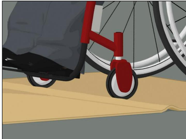
Exposed edges must have trim on the entire length of the exposed edge and be fastened to the floor to prevent curling. Trim must meet specifications for changes in level, including requirements for beveled edges when the height exceeds 1/4 inch. The maximum height is 1/2 inch.
